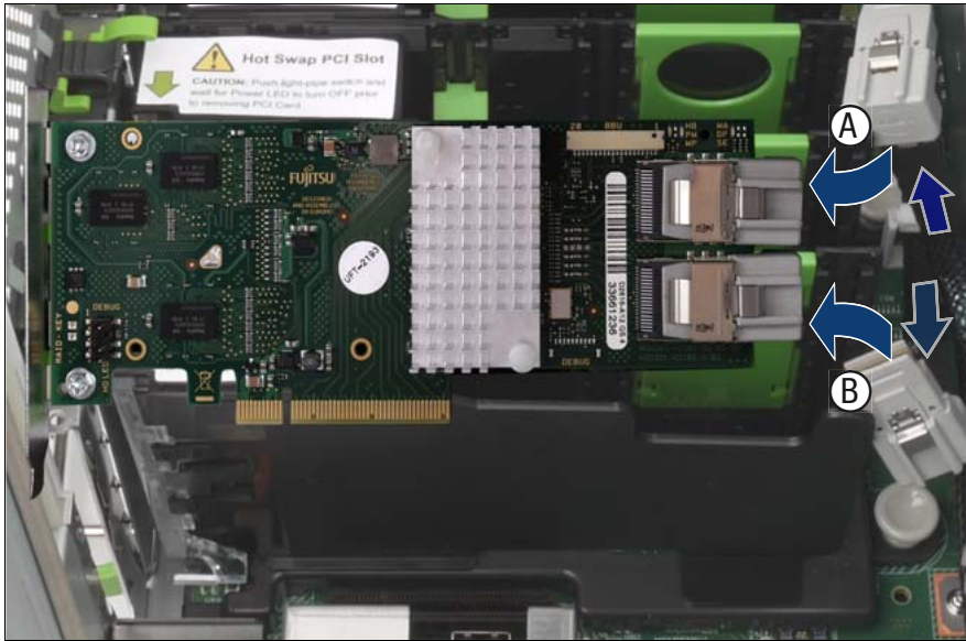
Figure 96: Connecting the SAS cables
